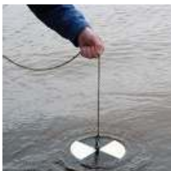
FIGURE 53. Example of a Secchi disc used for measuring water clarity.
